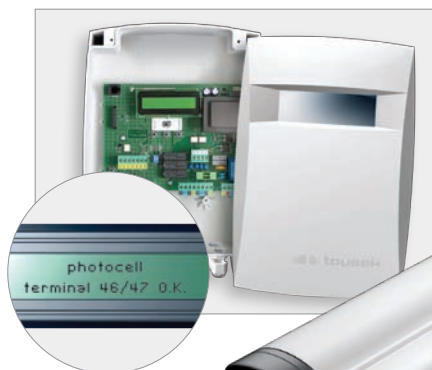
The control ST 12/4 with display and clear text menus
