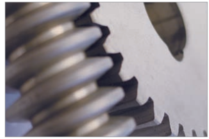
Motor and gears run in an oil bath and are therefore maintenance-free.
